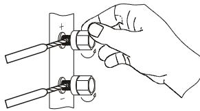
3. Tightening the copper post in clockwise direction, gently pull the wire, and make sure connection firmly.
